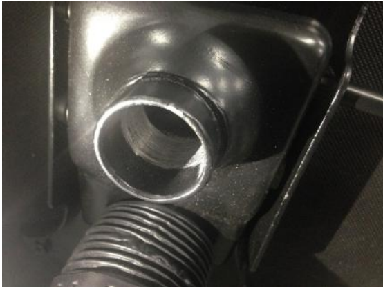
Photo No 7: Gas lift cone made in one piece
