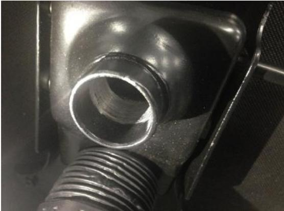
Photo No 7: Gas lift cone made in one piece
