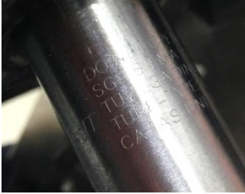
Photo No 5: Marking on the gas lift
